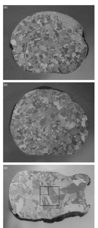
FIG. 5—Sequential cross-sections from Western Cartridge Company Mannlicher-Carcano lot 6000, bullet #2 (Pinkston notation), macro-etched to show grain size: (a) Pinkston section A; (b) Pinkston section E; and (c) Pinkston section I. Overlaid boxes in (c) depict 50-mg and 5-mg cubes. Section I was somewhat flattened during jacket removal. Original magnification  $\times$  14.
