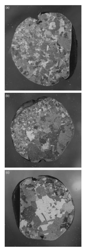
FIG. 6—Sequential cross-sections from lot 6000, bullet #8 (Pinkston notation), macro-etched to show grain size: (a) section A, (b) section E, and (c) section I. Original magnification  $\times 14$
