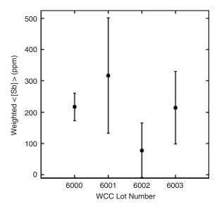
FIG. 1—Weighted-average [Sb] values of different lots of Mannlicher-Carcano 6.5-mm ammunition (data from (6)). Error bars are  $1\sigma$  confidence levels.
