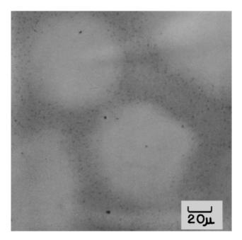
FIG. 3—Etched surface of a slowly cooled lead alloy, containing 100 ppm antimony, showing distribution of solid solution at dendritic boundaries. Elevated antimony areas etch darker. Grain size approximately 100 µm. From Simon and Jones (33), used by permission.
