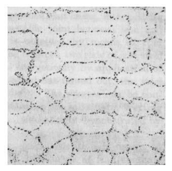
FIG. 4—Lead/400-ppm copper alloy, chill cast and nearly pure eutectic structure. The lead crystallized as dendrites, and copper precipitated at dendrite boundaries (dark areas). Original magnification  $\times$  150. From Hofmann (27), used by permission.
