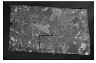
FIG. 7—Longitudinal cross-section from lot 6003, bullet #10 (Pinkston notation). Overlaid boxes depict 50- and 5-mg cubes. Original magnification  $\times$  10.9.
